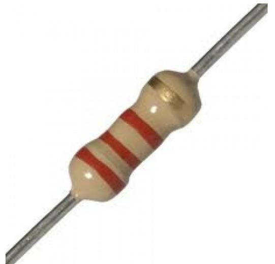
(k $\Omega$  Resistor 2.2)  $\times 1$
