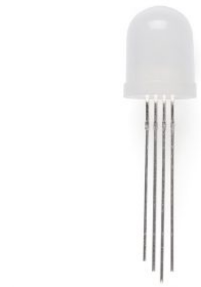
(10mm Common Cathode RGB LED) 1
