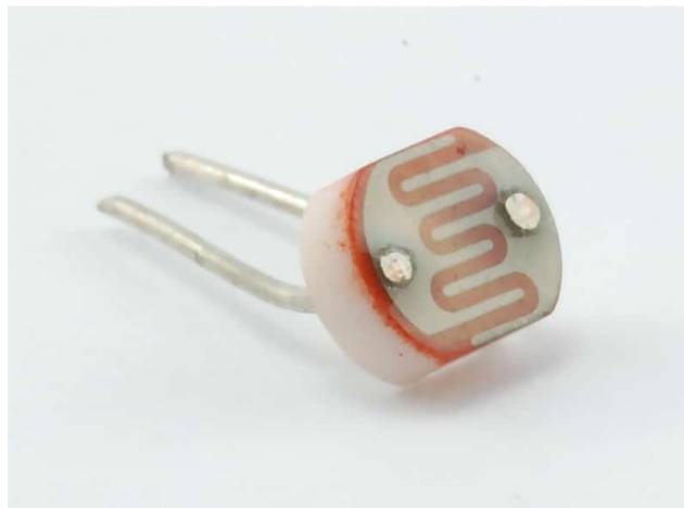
Light Dependent Resistor
