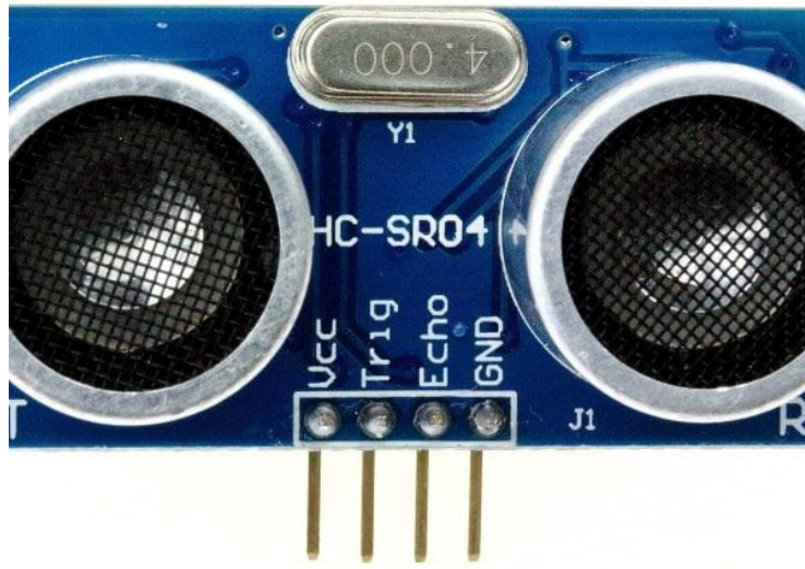
HC-SR04 Ultrasonic Sensor
