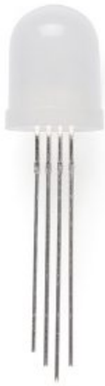
(10mm Common Cathode RGB LED) 1
