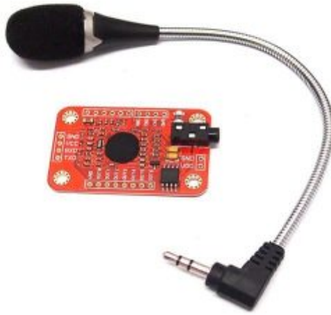
Voice Recognition Module v3
