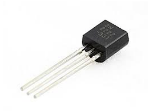
2n2222 NPN Transistor
