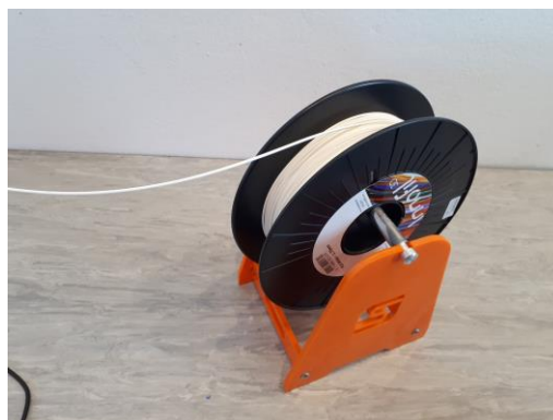
The filament roll holder is positioned so that the filament can unroll freely
